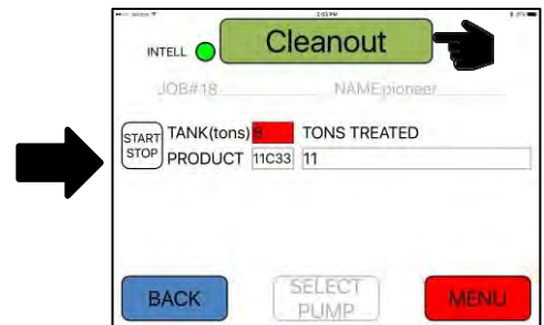
When keyed power has been off for 15 seconds, Cleanout begins automatically
